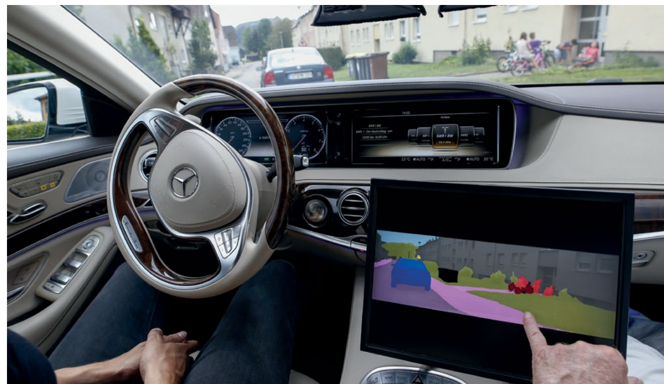
Children and parked cars are colour-coded on a monitor inside a Mercedes-Benz S-Class to make driving safer.
