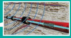
4 Acoustic-modulated light pulse is backscattered and recorded in the IU as VSP data.
